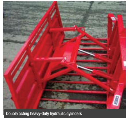
Double acting heavy-duty hydraulic cylinders
